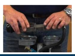
Install the two new gaskets onto the top of the valve plate.
