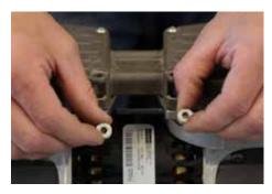
Reinstall the manifold using a 5/32" Allen wrench and the remaining two screws. Tighten the screws firmly to complete the installation (Recommended Torque: 47-50 in lb).
