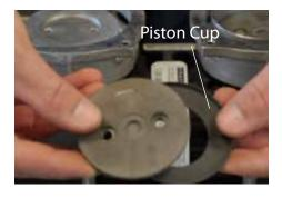
Place the retainer plate and and piston cup on top of the new piston cylinder sleeve. Flip over to ensure the piston cup is properly aligned within the cylinder sleeve.
