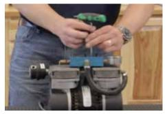
Remove the cylinder heads along with the valve plate and set to the side.
