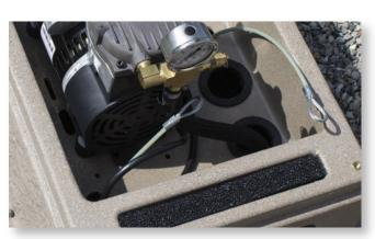
**Step 3:** Place cabinet on top of the galvanized stake and pass the security cable through two different grommet holes in the bottom of the cabinet.
