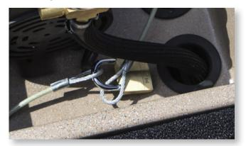
**Step 4:** Fasten the brass security lock to both ends of the security cable.
